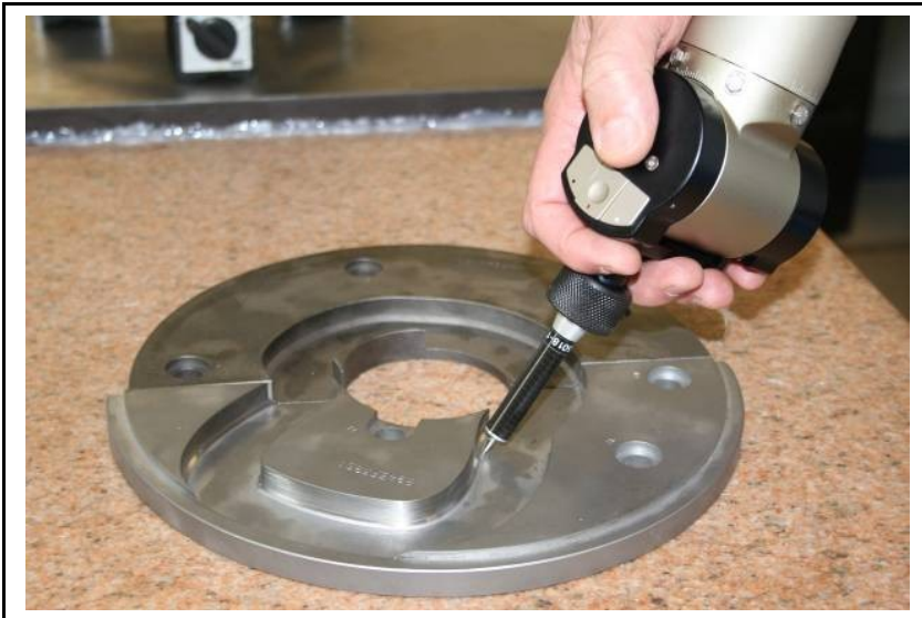
Figure 1: A PCMM is used at the front end of the cam reverse engineering process.
